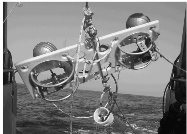
**Fig. 3.** Video camera system attached to top bridle prior to deployment. The high resolution, low light camera was placed on the right side of the mounting frame while the light source was on the left side. The pressure housing was hung beneath the frame.
