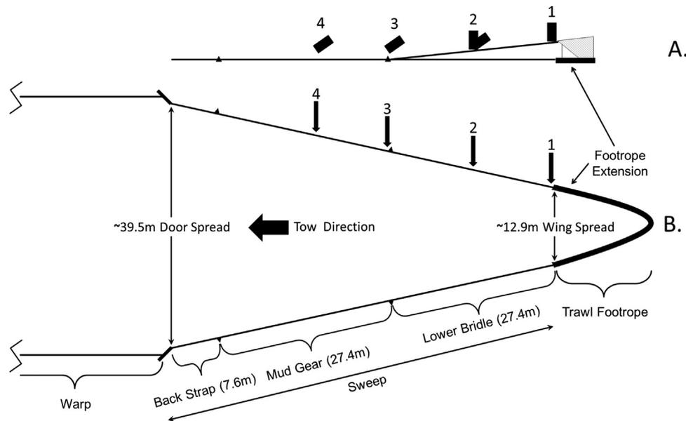
**Fig. 1.** Quasi-scale diagram of the Aberdeen-style trawl's footrope, bridles, mudgear, back strap, and doors under fishing conditions with indications of door and wing spread. The positions of the video camera system are marked with numerals 1–4.
